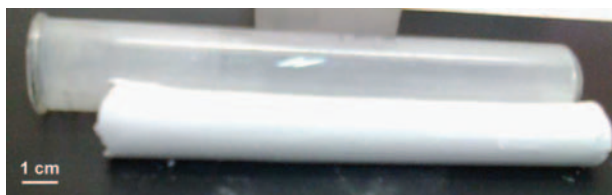
Fig. 4. Photograph showing the typical appearance of the synthesized monoliths of xerogels and aerogels.
